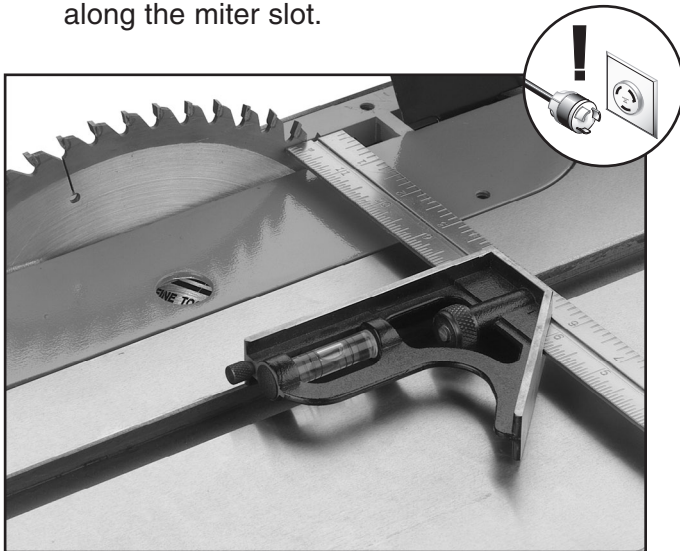
Figure 80. Example of adjusting blade to miter slot.
